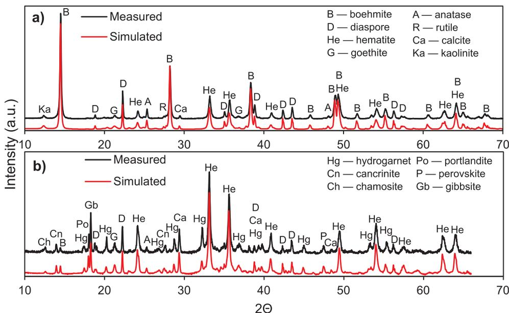
Fig. 1. Diffractograms and simulated patterns of (a) bauxite DD, and (b) bauxite residue.
