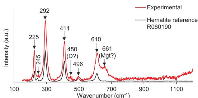
Fig. 3. Raman spectrum of an example hematite matrix area of bauxite DD in relation to hematite reference. D — diaspre, Mgt — magnetite. Peaks with only numeric indexing are attributed to hematite. Reference spectrum is from RRUFF database, reprinted with permission from RRUFF project representative (Lafuente et al., 2015).
