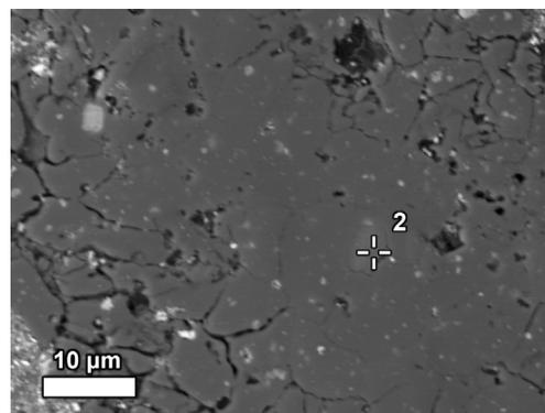
**Fig. 7.** Backscattered electron image of an aluminum oxyhydroxide dominant particle observed in bauxite residue. Quantification of spot “2” is shown in Table A.7.
