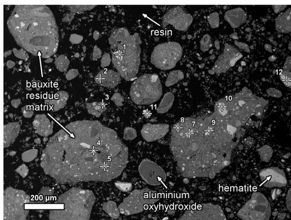
Fig. 4. Backscattered electron image of a selection of analyzed spots of hematite-dominant grains in bauxite residue. Measurements are summarized in Table 6 and individual measurements are reported in Table A.4.
