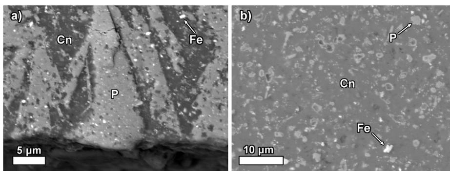
Fig. 10. Backscattered electron images of the Bayer process autoclave scale: (a) perovskite-enriched matrix, and (b) cancrinite-enriched matrix. Annotations: “P” — perovskite matrix, “Cn” — cancrinite matrix, “Fe” — iron oxide particle.
