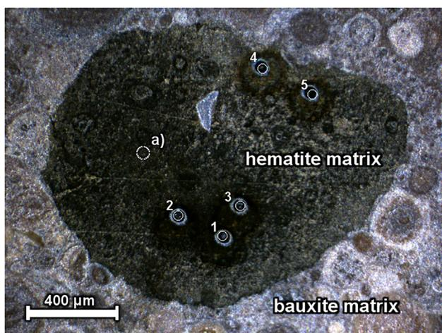
Fig. 2. Optical microscope image of bauxite DD hematite-dominant matrix area, surrounded by multiphase bauxite matrix. The numbers indicate LA-ICP-MS measurement spots (Table 5) and “a)” is the spot of  $\mu$ -Raman measurement depicted in Fig. 3.
