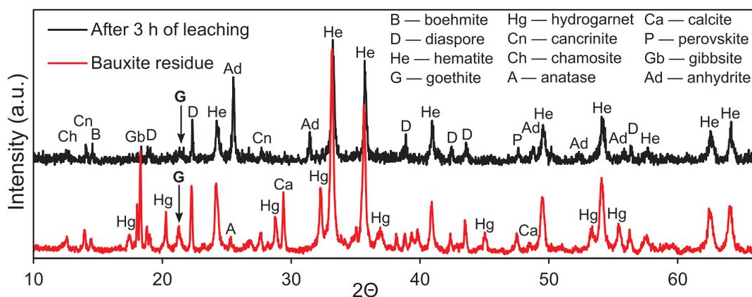
Fig. 11. Diffractogram of raw bauxite residue compared to diffractogram of residue after 3 h of leaching.
