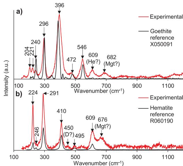
**Fig. 6.** Raman spectra of a) goethite area and b) hematite area contained in bauxite residue in relation to reference spectra. Analyzed locations are indicated on Fig. 5. He — hematite, D — diaspore, Mgt — magnetite; peaks with only numeric indexing are attributed to a) goethite, b) hematite. Reference spectra are from RRUFF database, reprinted with permission from RRUFF project representative (Lafuente et al., 2015).
