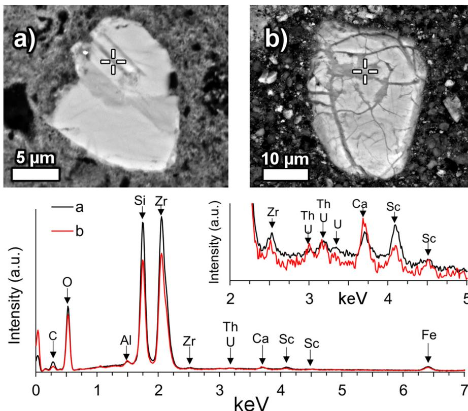
Fig. 8. Backscattered electron images of zircons observed in (a) Greek bauxite DD and (b) bauxite residue with respective EDS spectra.
