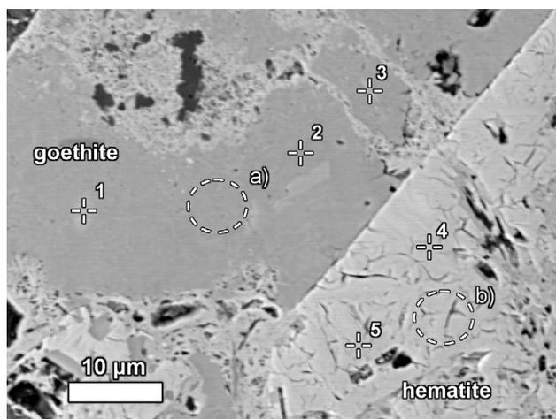
**Fig. 5.** Sc-rich goethite and Sc-depleted hematite contained in bauxite residue shown on backscattered electron image. Numbers 1 – 5 indicate to EPMA-WDS measurements (Table 7); letters “a)” and “b)” indicate the approximate areas of µ-Raman measurements (Fig. 6).
