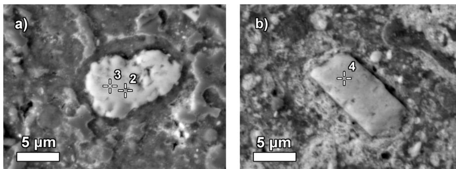
Fig. 9. Backscattered electron images of (a) titanium dioxide (anatase/rutile) and (b) iron titanate observed in Greek bauxite DD. The indicated quantification spots are reflected in (a) Table A.8 and (b) Table A.9.
