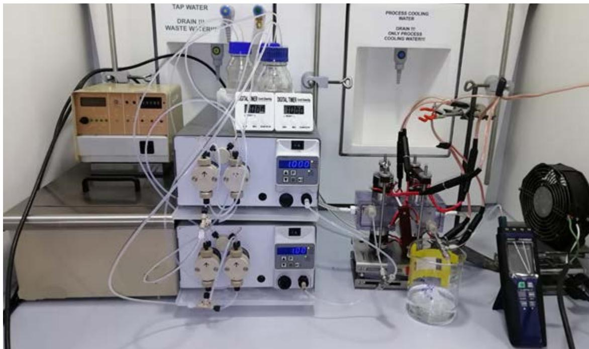
**Figure 2.** Photograph of the experimental setup. The polycarbonate reactor is connected to a heat transfer bath circulating silicon oil, HPLC pumps are used to deliver the reactants and a temperature sensor is connected to the reactor outlet. An air fan is used to cool the transducer temperature.
