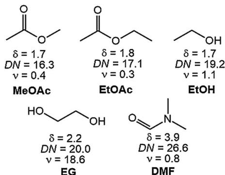
Fig. 2 Chemical structure, dipole moment  $\delta$ , in D, and Gutmann's donor number DN, in kcal mol<sup>-1</sup>, of methyl acetate (MeOAc), ethyl acetate (EtOAc), ethanol (EtOH), ethylene glycol (EG) and dimethylformamide (DMF).
