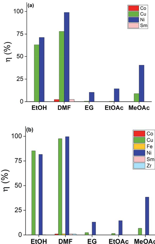
Fig. 3 Screening dissolution test for the SmCo<sub>5</sub> PMs (top) and Sm<sub>2</sub>Co<sub>17</sub> PMs (bottom) at 20 min in 1 vol% Br<sub>2</sub> in EG, DMF, EtOH, MeOAc and EtOAc. The recovery yields,  $\eta$  (%), were calculated as reported in eqn (1).
