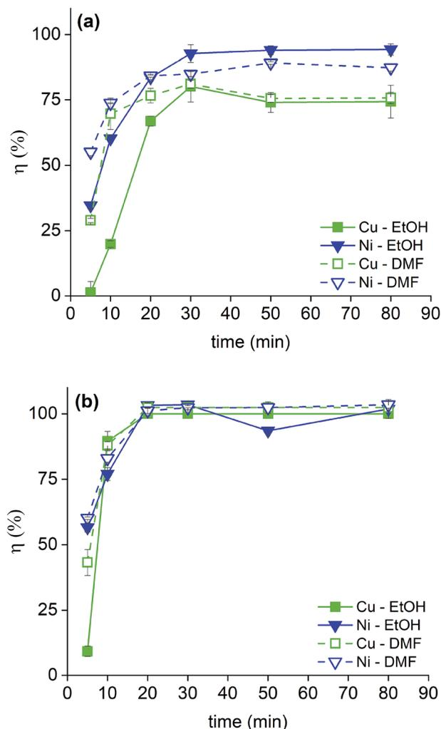
Fig. 5 Dissolution rate of the Ni–Cu–Ni coating of SmCo<sub>5</sub> PMs in 1 vol% Br<sub>2</sub> in EtOH and in 1 vol% Br<sub>2</sub> in DMF (a) and of the Ni–Cu–Ni coating of Sm<sub>2</sub>Co<sub>17</sub> PMs in 1 vol% Br<sub>2</sub> in EtOH and in 1 vol% Br<sub>2</sub> in DMF (b).
