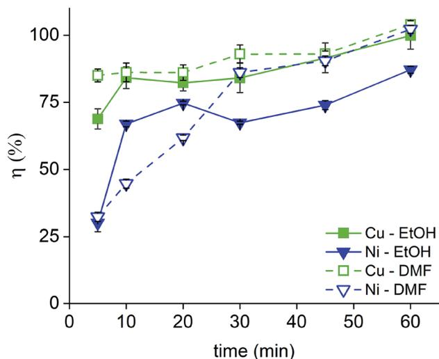
Fig. 4 Dissolution rate of the Ni–Cu–Ni coating of Nd–Fe–B PMs in 1 vol% Br<sub>2</sub> in EtOH and in 1 vol% Br<sub>2</sub> in DMF.
