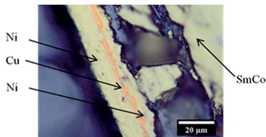
Fig. 1 Optical microscopy image of the three layers of Ni, Cu and Ni coating of a SmCo<sub>5</sub> magnet.
