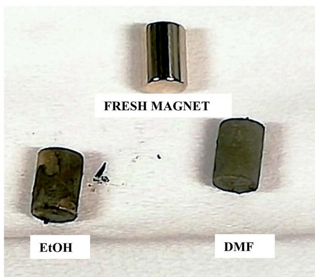
Fig. 7 Progressive removal of the metallic coating from Nd–Fe–B PMs by bromine–organic solvent mixtures.
