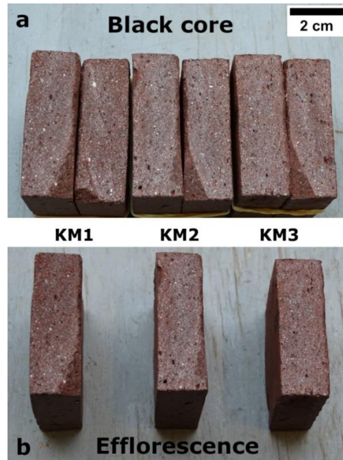
Fig. 4. Aesthetical properties of the paver mixtures fired at 1130°C (a) black core, (b) efflorescence.
