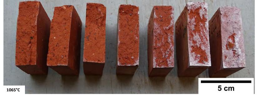
Efflorescence test result - Facing bricks
