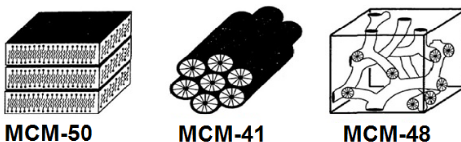
Figure 1.10. Schematic representation of the MCM materials: MCM-50 (layered), MCM-41 (hexagonal) and MCM-48 (Cubic). 114
