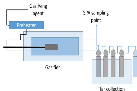
**Figure 1:** Fixed-bed gasifier.
