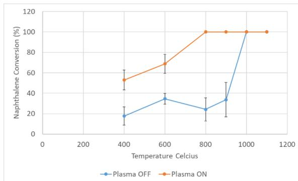
**Figure 5:** Naphthalene tar cracking using thermal-cracking only (blue line) and thermal-plasma cracking (red line)
