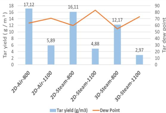
**Figure 4:** Tar yield and tar dew point in gasification experiments. Tar dew point is expressed in Celsius degrees.
