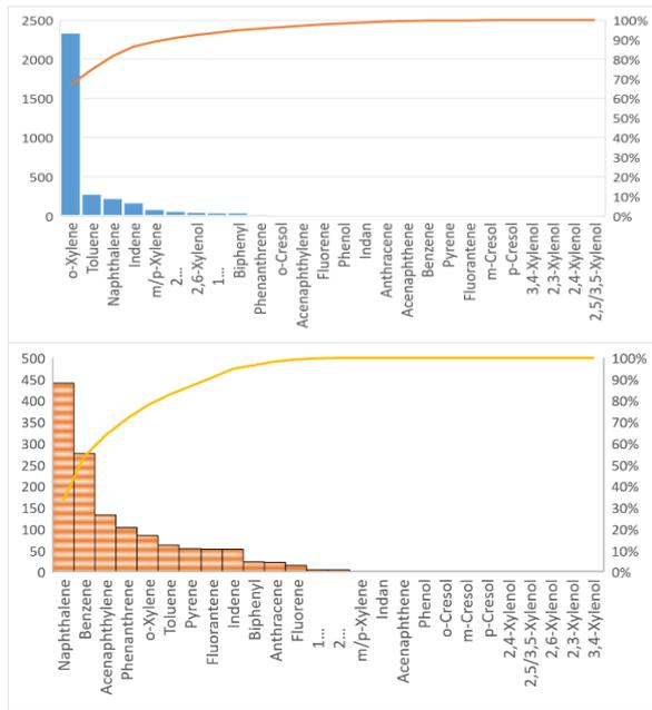
**Figure 3:** Tar composition for 3D MSW steam gasification. Concentrations are expressed in µg/100 ml Top: at 800°C, Bottom: at 1100°C
