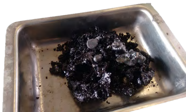
Figure 6. Sample 76 wt% BR, 5 wt% carbon, 9 wt% B 2 O 3 and 10 wt% silica, treated at 1200 °C (dimensions of the tray are 20 x 15 cm).
