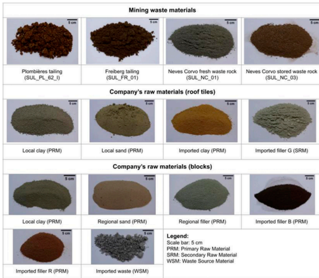
Fig. 2. Overview of the materials used to produce the ceramic mixtures after necessary pre-treatment.
