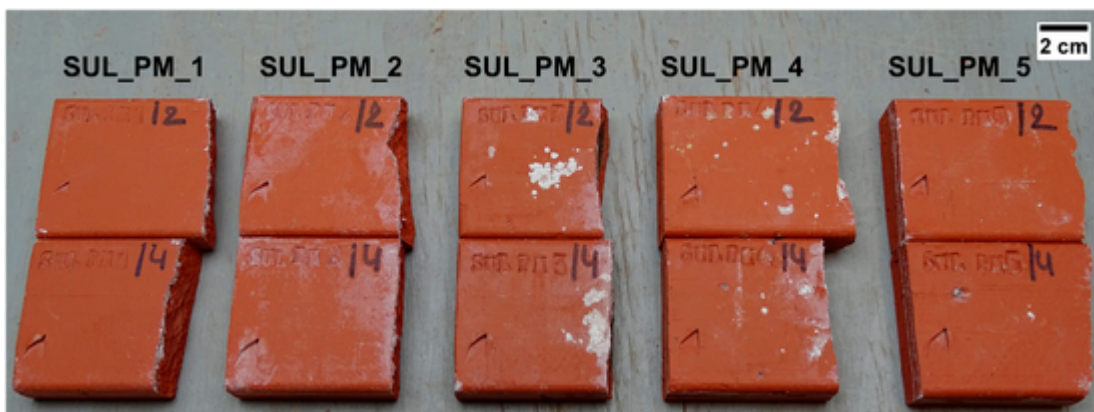
Fig. 7. Efflorescence test result on the fired roof tile test specimens (no. 12 fired at 985 °C and no. 14 fired at 1000 °C).
