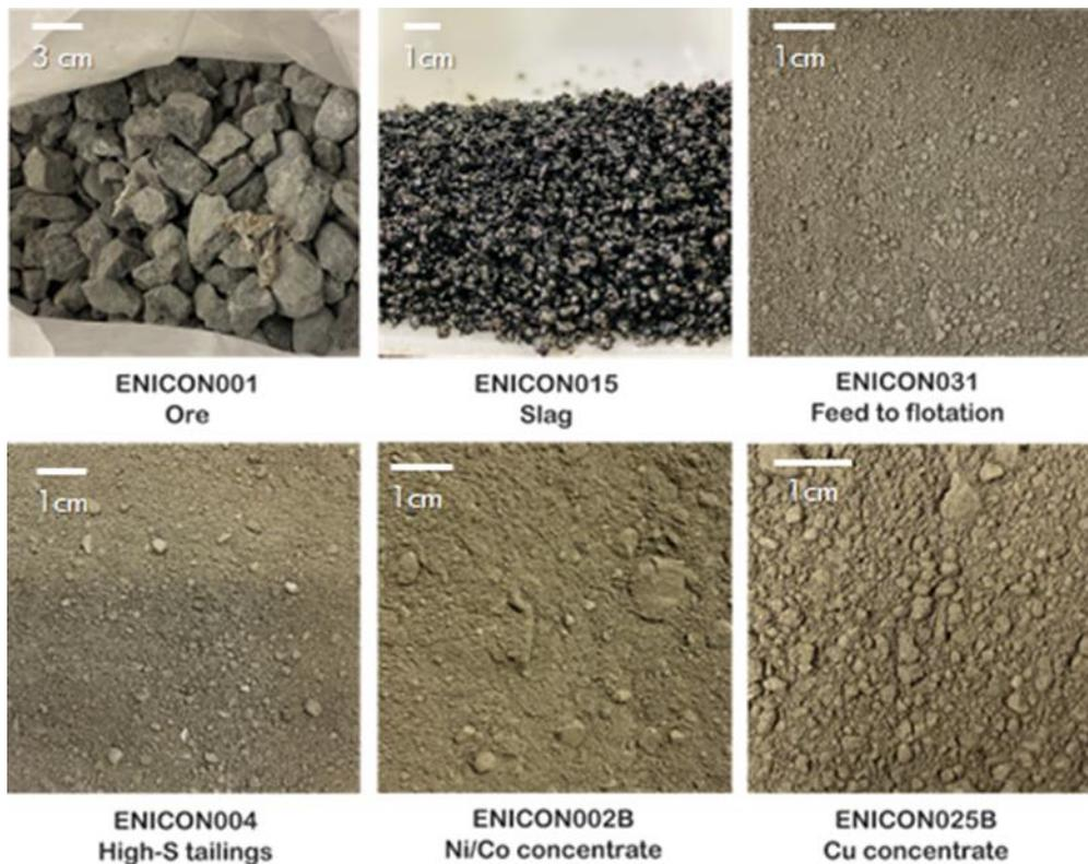
Figure 3. General aspects of some of the sulphide material samples studied, including the ore, slag, tailings, and concentrates.
